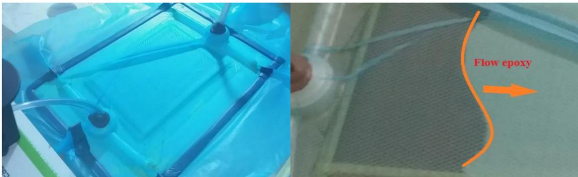
Fig. 2. Steps resin feed for manufacture laminated for DCB and ENF
