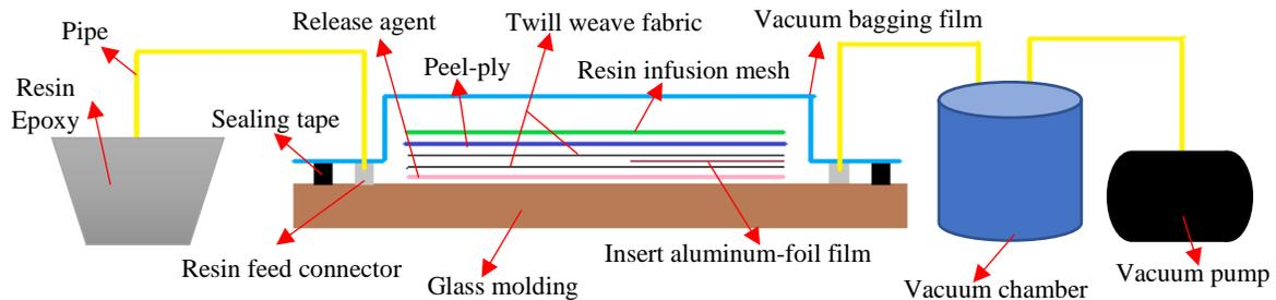
Fig. 1. SCRIMP technique was used to fabricate the pre-inserted CFRP panel
