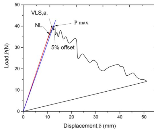
Fig. 9.  $G_{Ic}$  (Mode-I) load versus displacement representative curves
