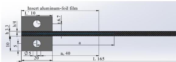
Fig. 4. Scheme in all dimensions according to ASTM for DCB Specimen
