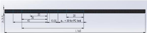
Fig. 5. Scheme in all dimensions according to ASTM for ENF Specimen
