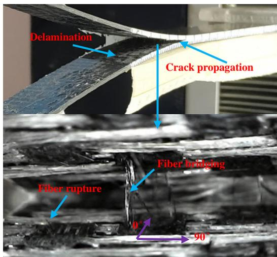
Fig. 10. Digital Microscope: fibers around the delamination zone (fiber bridging) during BCB
