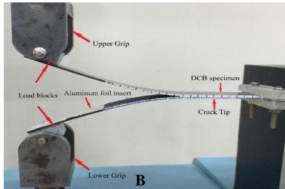
Fig. 6. DCB test: A) Magnifier was utilized to observe the growth delamination, B) During testing DCB specimens
