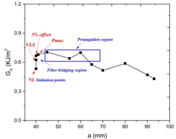
Fig. 11. R-curve, shown effect of fiber bridging on delamination onset and growth by MBT method
