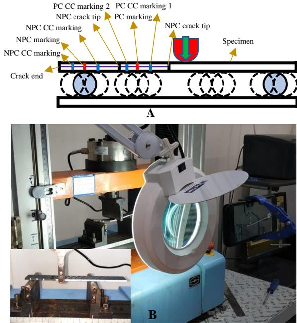
Fig. 7. Mode-II testing (a) Schematic, (b) Photograph of the ENF test setup
