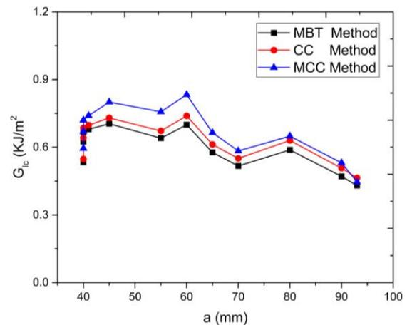
Fig. 12. R-curve, shown  $G_{Ic}$  calculation by three methods (MBT, CC and MCC)
