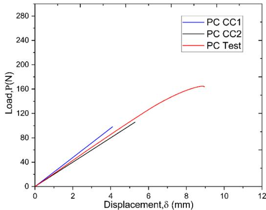
Fig. 16. Load- Displacement curves of the ENF PC test
