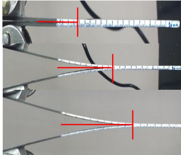
Fig. 14. Delamination length with increasing load
