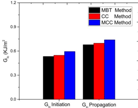
Fig. 13. Shown  $G_{Ic}$  initiation and  $G_{Ic}$  propagation value for methods (MBT, CC and MCC)
