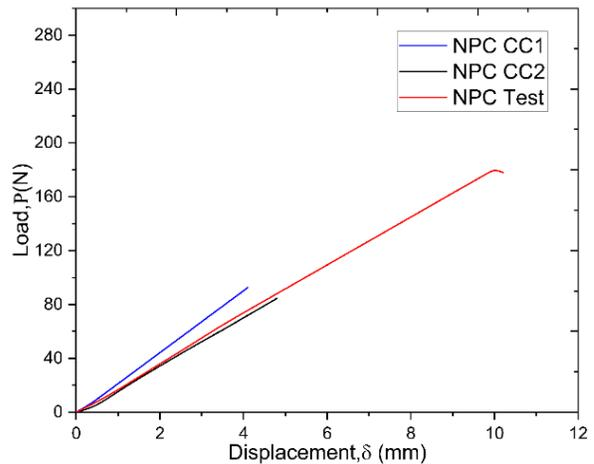
Fig. 15. Load- Displacement curves of the ENF NPC test
