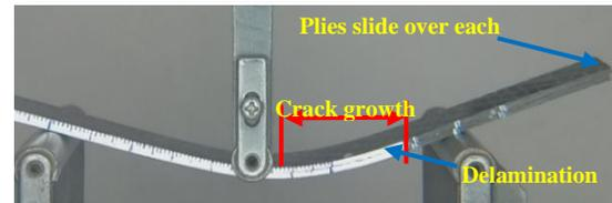
Fig. 17. Delamination growth during ENF test
