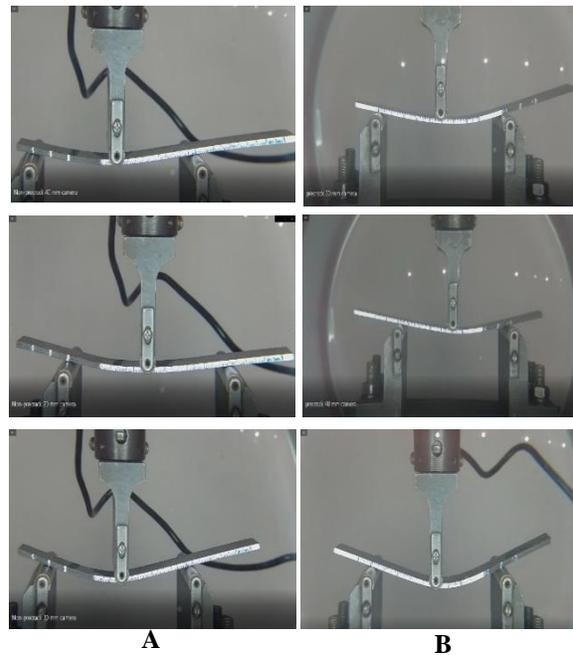
Fig. 8. Mode-II test. A) NPC specimen, B) PC specimen
